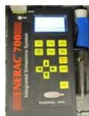
Students utilized an online Enerac 700 field portable emissions analyzer to take measurements of the boiler system used in the Six Points Brewery. This unit is the same unit that is used for the students when testing a Three Way Catalyst module in the unit operations laboratory sequence.
