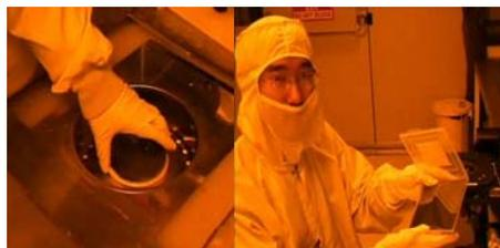
Figure 2: Samples from a micro-fabrication video demonstrating photo lithography techniques. The sample frames show how to create a thin photoresist layer on a Si wafer and use a mask alignment system.
