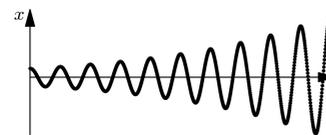
Use the forward-Euler approximation to make a discrete-time simulation of an undamped spring-mass system. Explain why the simulated position versus time (shown in the figure) so badly represents the behavior of an actual spring.
