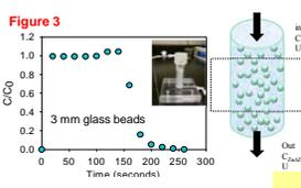
**Figure 3:** Where:  $C$  and  $C_0$  are the output and inlet bacterial concentrations,  $\theta$  is porosity,  $d_c$  is the collector diameter,  $\alpha$  is collision efficiency and  $\eta$  is collector efficiency and  $L$  is the column height.
