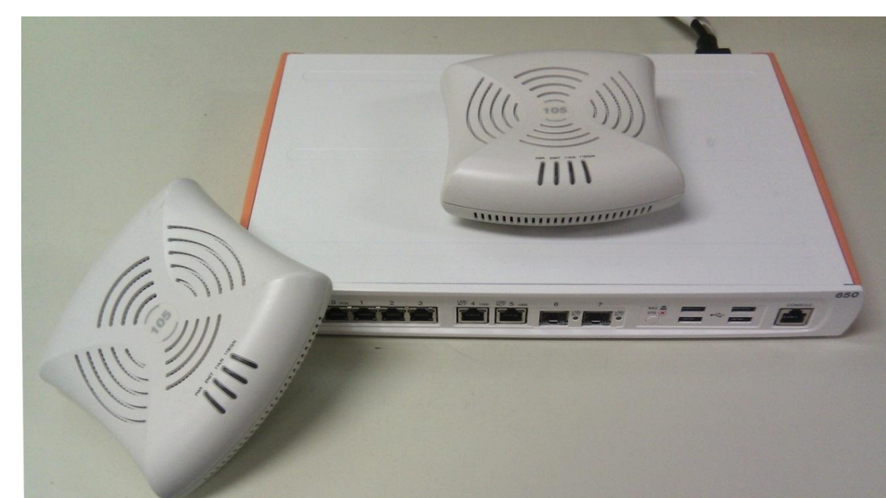
Aruba Networks controller and access points
